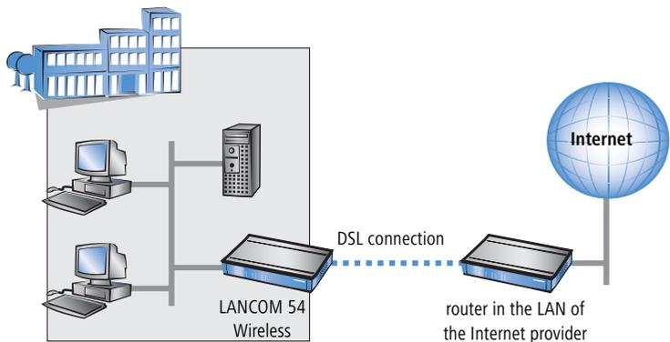
The task of a LANCOM 54 Wireless is to transfer data from the local network to the target network via a suitable WAN connection. Data is also transferred from the WAN to the desired recipients in the LAN.
