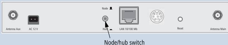
The node/hub switch is always in position 'node', when the LANCOM 54 Wireless base station is connected to a network. The setting 'hub' is needed, when the base station will be directly connected to another device like a single PC or a DSL modem.
