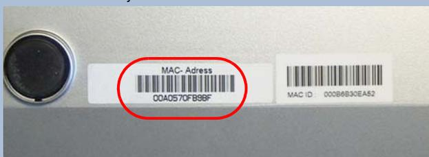
A device with the LAN MAC address "00A0570FB9BF" thus has a standard WEP key of "L00A0570FB9BF". This key is entered into the 'Private WEP settings' of the device for each logical WLAN network as 'Key 1'.
