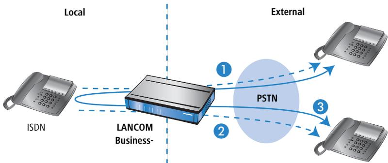
An ISDN telephone can transfer and interconnect the two active calls itself—even without a PBX. The ISDN telephone connects the two calls with each other internally and the two callers can speak with one another directly. The disadvantage of this variant is that the two lines which would normally be available on the ISDN telephone are both engaged. The user who connected the two callers can no longer conduct calls and is not able to receive calls for as long as the other two continue their call.
