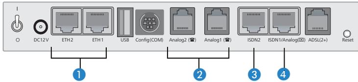
① **Connecting to the LAN** – First of all connect your LANCOM Business-VoIP-Router to the LAN. Plug in one end of the supplied network cable (green connectors) to a LAN connector on the device ①, and the other end into an available network connector socket in your local network or a free socket on a switch or hub.
