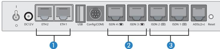
① **Connecting to the LAN** – First of all connect your LANCOM 1724 VoIP to the LAN. Plug in one end of the supplied network cable (green connectors) to a LAN connector on the device ①, and the other end into an available network connector socket in your local network or a free socket on a switch or hub.
