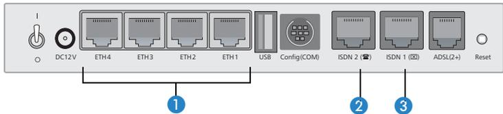
① **Connecting to the LAN** – First of all connect your LANCOM 1722 VoIP to the LAN. Plug in one end of the supplied network cable (green connectors) to a LAN connector on the device ①, and the other end into an available network connector socket in your local network or a free socket on a switch or hub.
