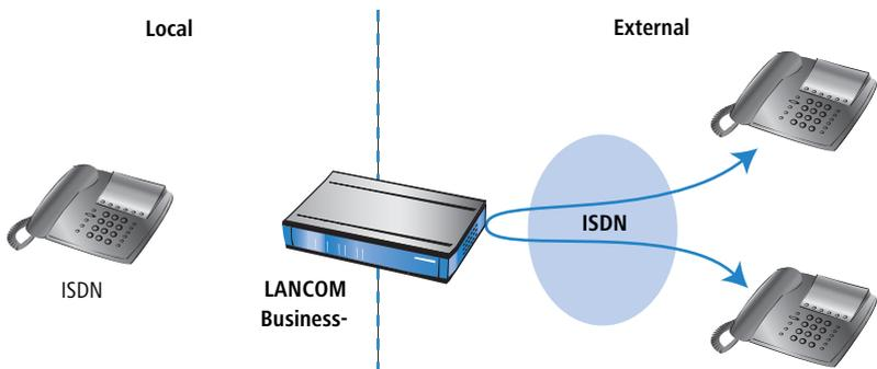
The disadvantage of this variant is that call forwarding blocks two ISDN channels in the LANCOM Business-VoIP-Router, even though none of the local users is making a call.
