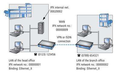
The three required network numbers are designated as "External Network Numbers" by the IPX conventions. Like IP network addresses, the apply to an entire LAN segment. On the other hand, internal IPX numbers are used to address specific Novell servers in the LAN. All three specified network numbers must be distinct from one another and from all used internal IPX network numbers.
