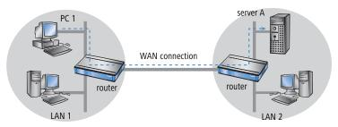
Connecting a LAN to the Internet does not technically differ from coupling two LANs. The only difference is that it is not just a handful of computers behind the Internet provider's router. Instead, it is the net of the networks - the public Internet.
