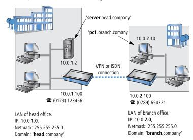
Unlike when accessing the Internet, all of the IP addresses in the involved networks are visible on the remote side when coupling networks, not just those of the router. The computer with the IP address 10.0.2.10 in the branch office LAN sees the server 10.0.1.2 in the headquarters and can access it (assuming it has the appropriate rights), and vice versa.
