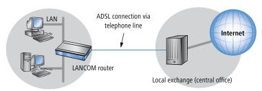
All DSL technologies, of which ADSL is the most common, are based on this concept. Thanks to their high transfer speeds, DSL connections are well-suited for Internet access.
