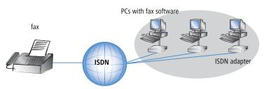
With LANCAPI by LANCOM it is possible to send faxes comfortably from your workstation PC, without having connected a fax device. To do so, you need to install several components:
