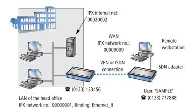
The required network numbers are designated as "External Network Numbers". Like IP network addresses, they apply to an entire LAN segment. On the other hand, internal IPX numbers are used to address specific Novell servers in the LAN. All three specified network numbers must be distinct from one another and from all used internal IPX network numbers.
