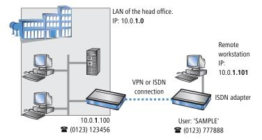
This IP address can be permanently assigned when setting up a user. However, it is simpler to let the LANCOM router automatically assign free IP addresses to users when they dial in. In this case you only need to specify the IP address range that the LANCOM router should use for RAS users.
