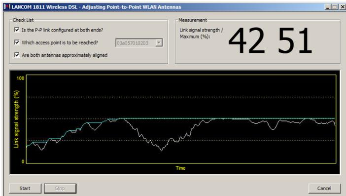
Initially only one of the two antennas should be adjusted until a maximum value is achieved. This first antenna is then fixed and the second antenna is then adjusted to attain the best signal quality.
