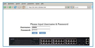
If you do not have the device's IP number, LANconfig can be used to search for it. To start LANconfig click on Start ➤ Programs ➤ LANCOM ➤ LANconfig.
