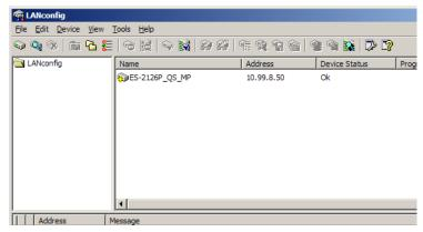
LANconfig automatically searches for all available devices in your network. Any available LANCOM devices will be displayed in the list, including the LANCOM switch. Double-click on this entry to start the browser automatically with the correct IP address.
