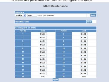
8191. As to port 25~port 26, only the fixed value "8192" is assigned to these two ports and user cannot configure this value.
