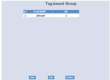
Add Group: Input the VLAN name, VID and then choose the member by ticking the check box beside the port No. to create a new Tag-based VLAN. As to the parameter of Untag, it stands for an egress rule of the port. If you tick the check box beside the port No., packets with this VID outgoing from this port will be untagged. Finally, press the <Apply> button to have the setting taken effect.
