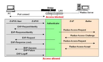
Only MultiHost 802.1X is the type of authentication supported in the switch. In this mode, for the devices connected to this port, once a supplicant is authorized, the devices connected to this port can access the network resource through this port.
