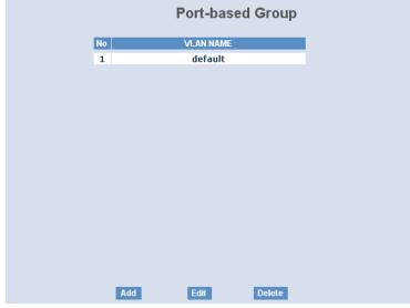
□ Add Group: Create a new Port-based VLAN. Input the VLAN name and choose the member by ticking the check box beside the port No., then, press the <Apply> button to have the setting taken effect.
