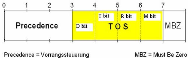
DiffServ DSCP Priority act on DSCP field of IP Header. In the late 1990s, the IETF redefined the meaning of the 8-bit SERVICE TYPE field to accommodate a set of differentiated services (DS). Under the differentiated services interpretation, the first six bits comprise a codepoint, which is sometimes abbreviated DSCP, and the last two bits are left unused.
