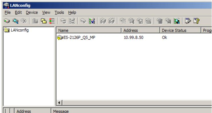
LANconfig automatically searches for all available devices in your network. Any available LANCOM devices will be displayed in the list, including the LANCOM switch. Double-click on this entry to start the browser automatically with the correct IP address.
