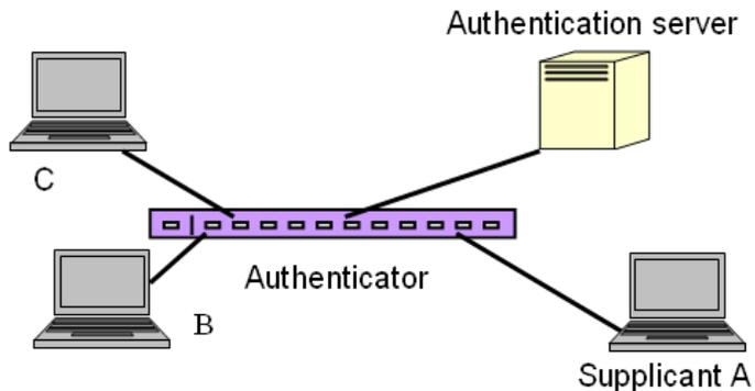
The figure shows the procedure of 802.1x authentication. There are steps for the login based on 802.1x port access control management. The protocol used in the right side is EAPOL and the left side is EAP.
