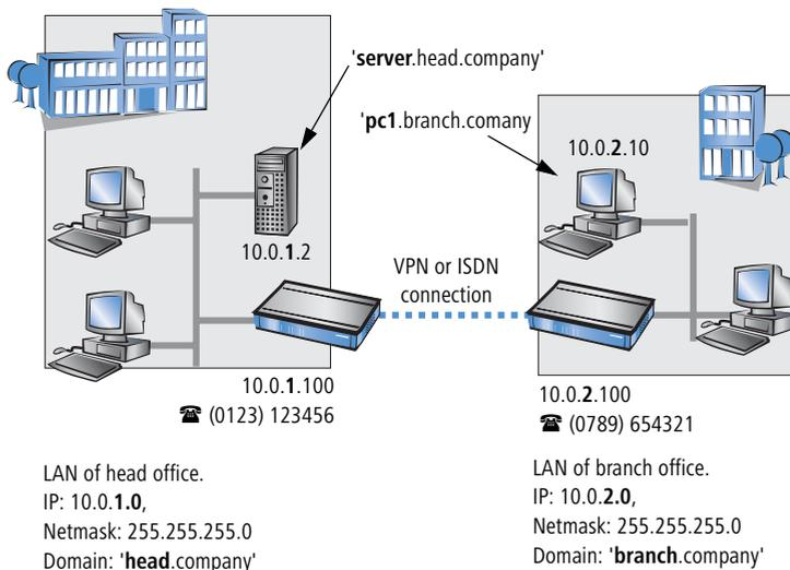
Unlike when accessing the Internet, all of the IP addresses in the involved networks are visible on the remote side when coupling networks, not just those of the router. The computer with the IP address 10.0.2.10 in the branch office LAN sees the server 10.0.1.2 in the headquarters and can access it (assuming it has the appropriate rights), and vice versa.
