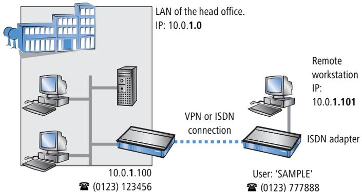
This IP address can be permanently assigned when setting up a user. However, it is simpler to let the LANCOM router automatically assign free IP addresses to users when they dial in. In this case you only need to specify the IP address range that the LANCOM router should use for RAS users.
