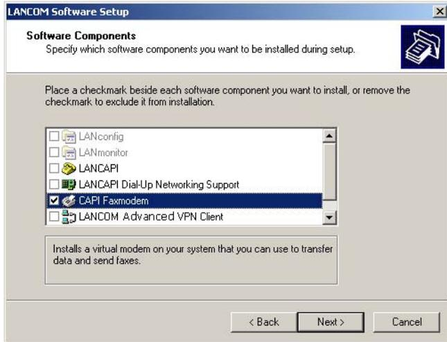
When the installation was successful, the LANCOM **CAPI fax modem** is entered into the **Phone and Modem Options** of the control panel.
