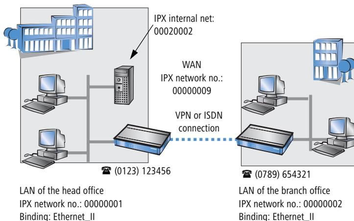
The three required network numbers are designated as “External Network Numbers” by the IPX conventions. Like IP network addresses, they apply to an entire LAN segment. On the other hand, internal IPX numbers are used to address specific Novell servers in the LAN. All three specified network numbers must be distinct from one another and from all used internal IPX network numbers.
