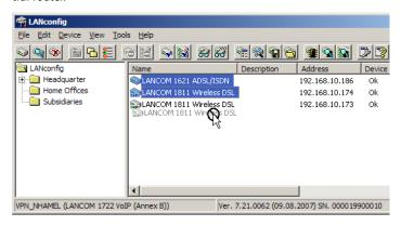
3 The 1-Click-VPN Site-to-Site Wizard will be started. Enter a name for this access and select the address under which the router is accessible from the Internet.
