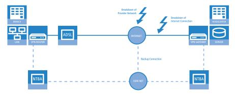
IPSec-based VPN provides optimal security for connecting branch offices and home offices thanks to the high-security 3-DES or AES encryption, integrated hardware acceleration, and support of digital certificates.
