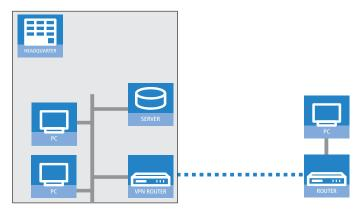
This IP address can be manually set to a fixed value when the user is created. A simpler option is to allow the LANCOM Router to assign the user with a free IP address when dialing in. In this case, all you have to do is to set the range of IP addresses which are to be available for assignment to the RAS users by the LANCOM Router.
