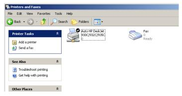
To check the installation, click with the right-hand mouse key on the fax icon and select **Properties**. The LANCOM CAPI Faxmodem should be entered on the 'Devices' tab.
