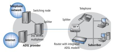
In some models (like in the picture above) the ADSL modem is integrated directly in the router (e.g. LANCOM 821 ADSL/ISDN and LANCOM 1621 ADSL/
