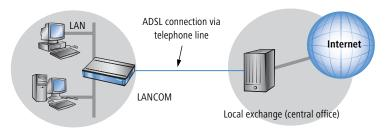
All DSL technologies, of which ADSL is the most common, are based on this concept. Thanks to their high transfer speeds, DSL connections are well-suited for Internet access.
