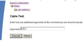
Change then to menu item **Expert configuration** ➤ **Status** ➤ **LAN statistics** ➤ **Cable test results**. The results of the cable test for the individual interfaces are show up in a list.
