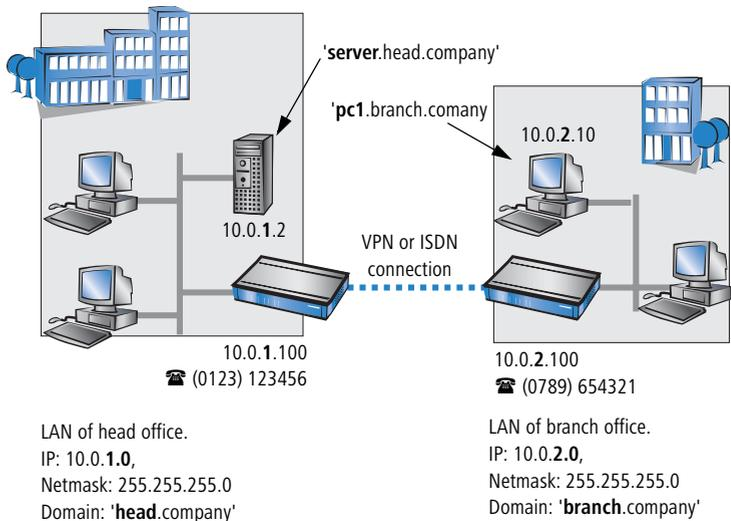
Unlike when accessing the Internet, all of the IP addresses in the involved networks are visible on the remote side when coupling networks, not just those of the router. The computer with the IP address 10.0.2.10 in the branch office
