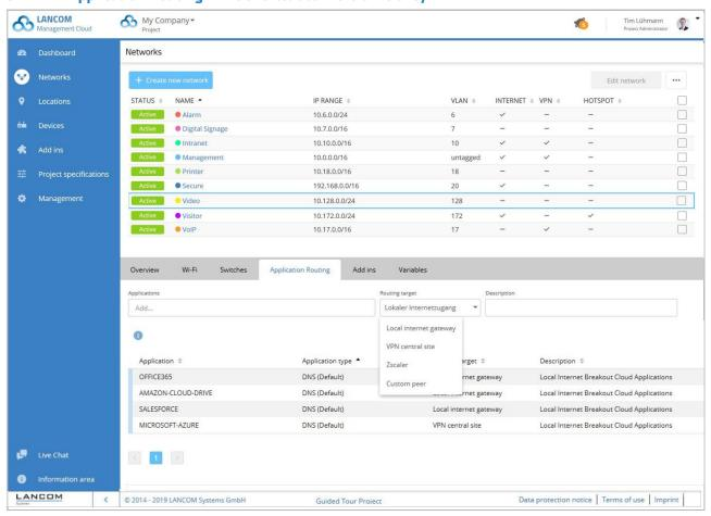
Benefit from significant performance gains when you operate modern cloud applications (e.g. Office 365, Sales-Force, etc.). SD-WAN Application Routing detects cloud-based applications and routes them directly to the Internet (local break-out). This boosts your cloud applications and relives the VPN path to the headquarters as well as the headquarter's Internet line.
