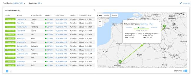
Performance monitoring can be activated in the configuration dialog for each network. The monitoring target for the measurement is also defined there, allowing individual and flexible quality monitoring. Note: Performance monitoring is supported by all LANCOM VPN Gateways as of LCOS 10.30.
