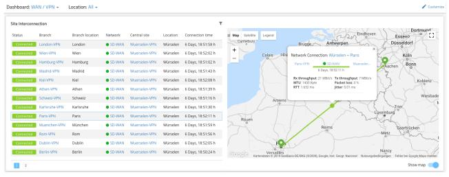
Performance monitoring can be activated in the configuration dialog for each network. The monitoring target for the measurement is also defined there, allowing individual and flexible quality monitoring. Note: Performance monitoring is supported by all LANCOM VPN Gateways as of LCOS 10.30.
