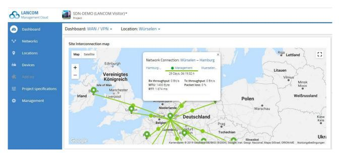
For this, VPN Performance Monitoring can be enabled per network in the network configuration, and the endpoint for the measurement can be specified. A firmware version LCOS 10.30 or newer is required.
