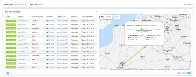
Performance monitoring can be activated in the configuration dialog for each network. The monitoring target for the measurement is also defined there, allowing individual and flexible quality monitoring.
