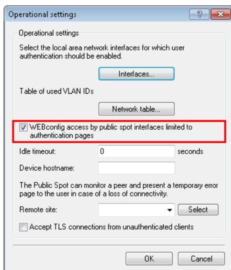
! Note that using permissions under **Management > Admin > Configurations access ways > Access rights** you cannot generally limit the access via HTTP(S) to the device.
