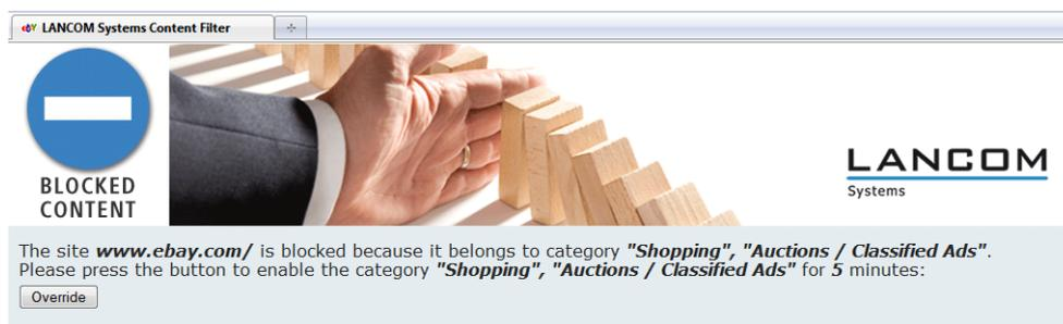
In case of an override, the content filter displays the relevant entry from the block-text table and directly below this, the text from the override-text table together with the 'Override' button. When the user clicks this button the content filter forwards the user to the requested page, if possible. If it is not possible to forward the user to the requested page, the content filter displays an error page.
