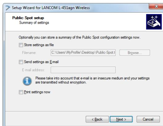
**12. The click **Next** and finally **Finish** to complete the basic installation of the Public Spot. The Setup Wizard will now send the settings to the device.**
