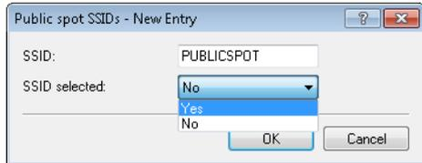
The Create Public Spot account wizard automatically marks the specified network names as **SSID selected** when creating a new Public Spot user. If you employ an access point or WLAN controller, you are able to select several network names as default values in order to give users access to different WLANs. When creating a new user and subsequently printing the voucher, these SSIDs are also printed out on the voucher.
