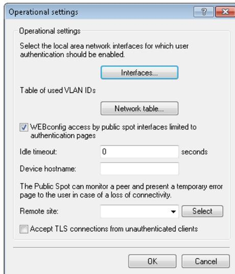
To enable the HTTPS redirect, activate the option **Accept TLS connections from unauthenticated clients**. This option is disabled by default.
