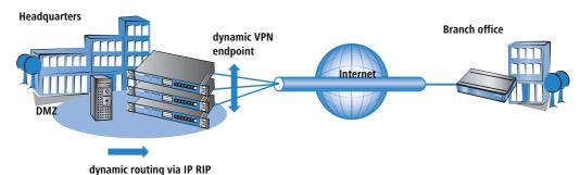
In decentralized company structures that rely on VPN for networking the various locations, the availability of the central VPN gateway is of particular significance. The company-wide communications only remain reliable as long as these central dial-in nodes are working properly.
