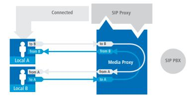
In this case it is not necessary to pass the media streams through the upstream PBX, so the SIP signaling helps the LANCOM VoIP Router to make a new decision on the path to be taken by the connection data. Using the end points in the media proxy the data streams can be connected directly, making a diversion via the SIP PBX unnecessary.
