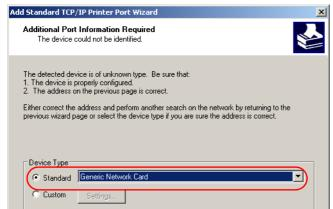
(6) Alternatively, you can select 'Custom' and press on the **Settings** button to open an additional dialog. In this dialog, you can select the protocol to be used for transmitting the print jobs to the printer at the USB port of the LANCOM ('Raw' for RawIP or 'LPR').. The port to be used can be entered here too (for RawIP only). For LPR, port '515' is always used as standard.
