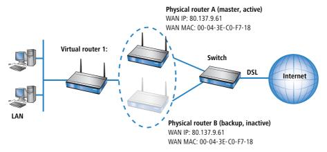
Due to the fact that the LANCOM terminates its WAN connection when the last virtual router switches to backup mode, this requirement is definitely fulfilled when a total of only one virtual router has been defined.
