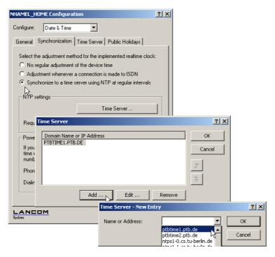
With these settings only the LANCOM applies the time from public time servers. To provide the real time for the remaining device enable the local time server under the tab 'Time Server'. Furthermore activate the broadcast mode and enter the broadcast interval.
