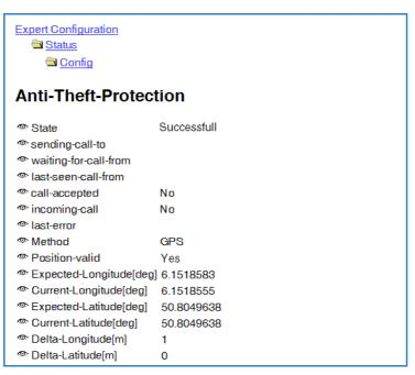
Only when the location verification has the status 'Successful' will the router data be transferred over the WAN interfaces.
