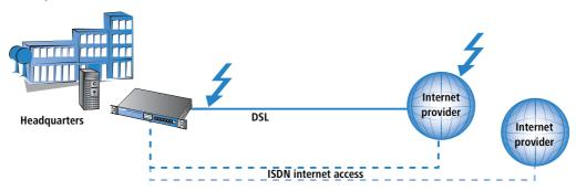
In this simple backup scenario, Internet access is realized via a DSL connection. An ISDN connection is defined as a backup in case of failure of the DSL Internet access.
