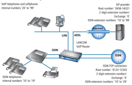
In this example we will take a look at a company planning to add a SIP trunking account, with up to 100 extension numbers, to its current ISDN point-to-point line having 20 extensions. The ISDN terminal devices with point-to-point
