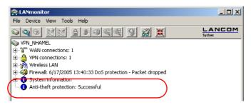
With WEBconfig (Expert configuration > Status > Config > Location verification) or Telnet (Status/Config/Location verification) you can view the status of the location verification:
