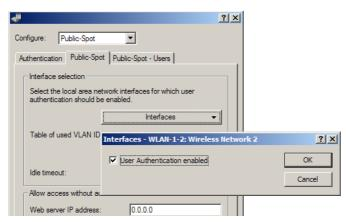
Activating the authentication for a WLAN interface automatically enters the associated SSID into the temporary public-spot accesses.
