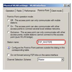
In the point-to-point configuration, select the identification by station name and enter the name of the corresponding station.
