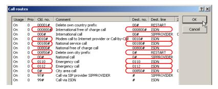
(5) In order to allow the ISDN subscribers to be contacted internally by the VoIP users, a standard route is also set up which directs all calls that have not yet been resolved to the ISDN line without changing the numbers.
