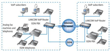
Along with data transfer via VPN, it is also possible to use VoIP functions between the two locations.
