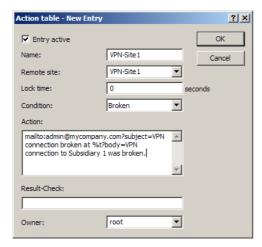
Select the remote site for the relevant connection. As Condition select 'Broken' and enter the action as the transmission of an e-mail.
