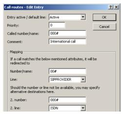
After being adapted, the call routing table should appear as follows:
