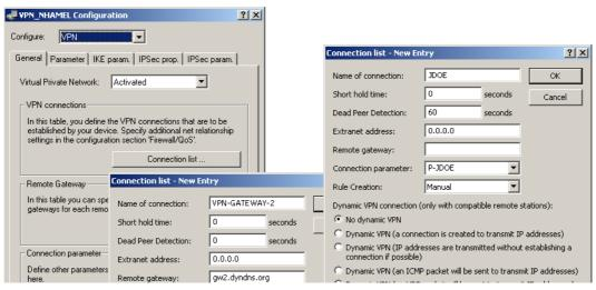
Configuration with WEBconfig, Telnet or SSH Under WEBconfig, Telnet or SSH client you will find the settings for the dead peer detection under the following paths:
