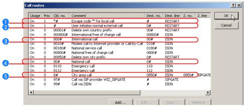
The other routes are used to carry out international 3 and national 4 long distance calls as well as local calls 5 as standard over the ISDN line. The Call Router removes the preceding zeros from the number again and sends the call out to the ISDN line.
