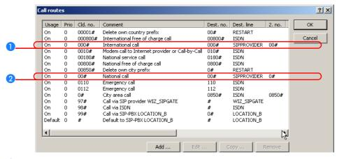
① In this state, all calls that cannot be resolved by the call routing table and which do not have a corresponding entry in the local user list are automatically forwarded to the remote site.
