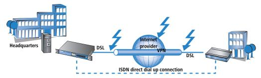
In the case that a branch office is connected to the headquarters via a VPN connection, the Internet-based VPN connection can be backed up by a direct ISDN dial-in connection. Should the Internet connection fail at either of the two routers, the data transmission is transferred to the ISDN link.
