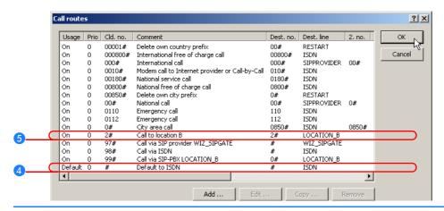
This entry for 'LOCATION\_B' is placed well down toward the end of the call routing table so as not to affect the more general rules. However, for interaction with the other routes, verify that only the internal numbers for the remote site are directed to the respective line.
