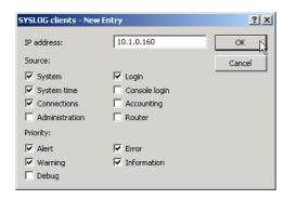
SYSLOG comes from the UNIX world, in which specified sources are predefined. LANCOM assigns its own internal sources to these predefined SYSLOG sources, the so-called "facilities".
