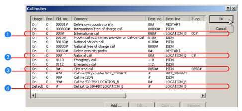
6 Adapt the suggested call routing table in order to make international and national long distance calls via the SIP provider line with backup over ISDN. When doing so, please observe that the '0' preceding the number must be removed.
