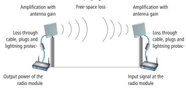
1 The calculation of the power over the path begins at the transmitters's radio module. The radio module in the LANCOM access points in 802.11a mode emits the following power levels depending on the channel used and the data transmission rate:
