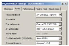
You can find these parameters in WEBconfig or Telnet under **Expert Configuration** ▶ **Setup** ▶ **Interfaces** ▶ **WLAN** ▶ **Radio Settings**.
