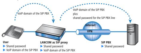
If SIP or ISDN users at the LANCOM VoIP Router are entered into the SIP PBX with different passwords, then the users have to enter their individual passwords upon registration. Consequently, each SIP or ISDN user has an entry into the LANCOM with the individual passwords, which are also entered into the SIP terminal devices. Users with shared and individual passwords can be managed in parallel.
