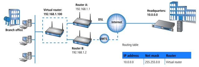
From a more technical standpoint, a router in a network requires a unique MAC address in addition to an IP address. Therefore, when defining a virtual router, a virtual MAC address is defined simultaneously which the virtual router reacts to. The virtual MAC address is formed as '00-00-54-00-01-xx', whereby 'xx' stands for the unique router ID.
