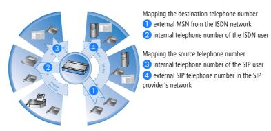
Depending on the application at hand, both the called and the calling numbers have to be modified so that a return call can be made to the source number.
