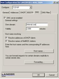
Activated DNS server in the TCP IP configuration
