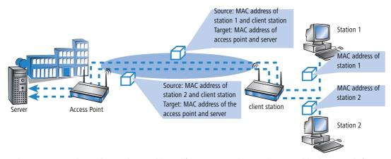
In this operating mode not the usual MAC addresses for instance in client mode are used (in this example for server, access points and client stations), but in conformity to point-to-point connections four addresses (the MAC address
