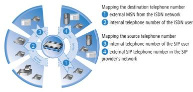
Depending on the application at hand, both the called and the calling numbers have to be modified so that a return call can be made to the source number.
