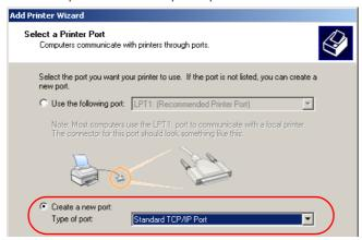
4 Enter the IP address of the LANCOM as the IP address of the printer port. The name for the printer port will automatically be filled out with 'IP\_<IP address of the LANCOM>'.
