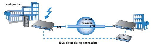
Going a step further, the VPN gateways themselves can be backed up in case of failure. This case assumes the existence of a VPN connection between two gateways. In the event that one of the two VPN devices should fail, an ISDN connection is to take over the data transfer; in this case via a direct dial-in connection.
