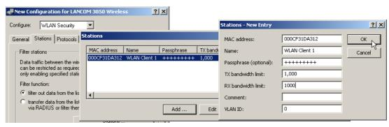
Configuration with WEBconfig, Telnet or SSH Under WEBconfig, Telnet or SSH client you will find the MAC access list under the following paths:
