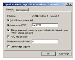
Closed network mode You can operate your wireless LAN either in public or private mode. A wireless LAN in public mode can be contacted by any mobile station in the area. Your wireless LAN is put into private mode by activating the closed network function. In this operation mode, mobile stations that do not know the network name (SSID) are excluded from taking part in the wireless LAN.
