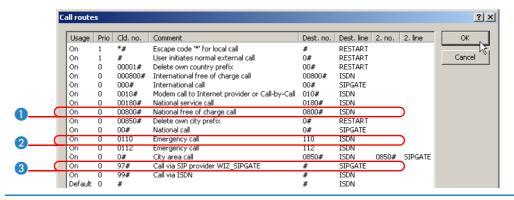
This call routing table is only valid for PBX systems that forward the special character star '\*' for internal calls on their external ISDN bus. If the PBX processes this character in a different manner, then the table must be adapted accordingly.
