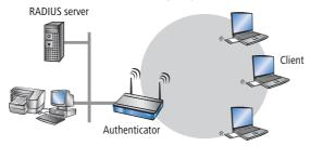
Authentication server: RADIUS server on which user data is configured. This is usually located within the same network for which it issues access authorizations. It is accessible to the client via the authenticator. Some scenarios may also allow the use of a LANCOM access point for this task.
