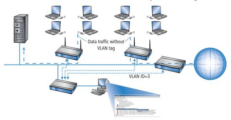
By setting up a virtual LAN between the base stations and the administrator's switch, management data is shielded against all "public" traffic on the LAN.
