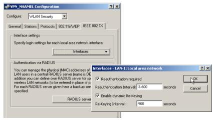
Configuration with WEBconfig or Telnet Under WEBconfig or Telnet you will find the settings for IEEE-802.1x under the following paths:
