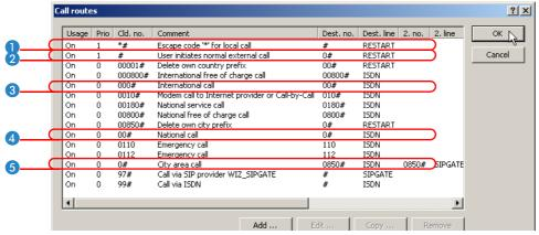
The other routes are used to carry out international 3 and national 4 long distance calls as well as local calls 5 as standard over the ISDN line. The Call Router removes the preceding zeros from the number again and sends the call out to the ISDN line.
