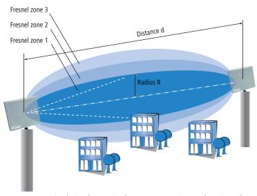
To ensure an optimal signal reception between transmitter and receiver, the Fresnel zone 1 should remain free from any obstruction. Any disturbances from elements protruding into this zone will significantly reduce the effective signal power. The object not only screens off a portion of the Fresnel zone, but the resulting reflections also lead to a significant reduction in the signal reception.
