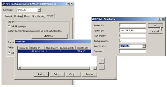
Configuration with WEBconfig, Telnet or SSH Under WEBconfig, Telnet or SSH client you will find the settings for VRRP under the following paths:
