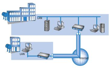
A VPN-enabled router (VPN gateway) is located at either end of the tunnel. The configuration of both VPN gateways must be matched to one another.
