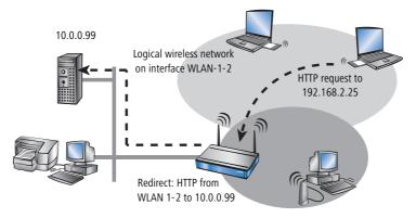
All requests with this protocol from this logical wireless network will automatically be redirected to the target server in the LAN. The returning data packets are sent to the senders' addresses and ports according to the entries in the connection statistics, which ensures the trouble-free operation in both directions. Further information to the configuration of the protocol filter can be found 'Protocol filter'  $\rightarrow$  page 379
