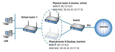
Due to the fact that the LANCOM terminates its WAN connection when the last virtual router switches to backup mode, this requirement is definitely fulfilled when a total of only one virtual router has been defined.
