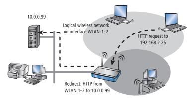
All requests with this protocol from this logical wireless network are automatically redirected to the target server in the LAN. The returning data packets are sent to the senders' addresses and ports according to the entries in the connection statistics, ensuring trouble-free operation in both directions.
