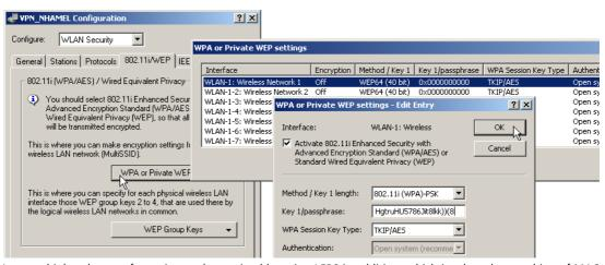
An even higher degree of security can be attained by using LEPS in addition, which involves the matching of MAC address and passphrase. When using LANconfig for the configuration, you enter the passphrases of the stations approved for the WLAN in the configuration area 'WLAN Security' on the 'Stations' tab under the button **Stations**.
