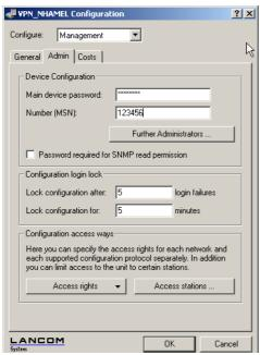
2 Enter a number (MSN) at your location which is not being used for other purposes in the 'Device Configuration' area.
