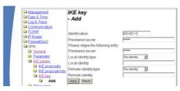
② Under Configuration ➤ VPN ➤ General ➤ Connection parameters define a new "VPN layer" for the connection parameters. Select the IKE key created earlier for this.
