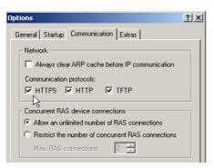
Using HTTP improves the transmission speed; HTTPS can also offer additional security mechanisms. The use of HTTPS is especially recommended for remote management over unsecured WAN connections (such as DYNDNS services).
