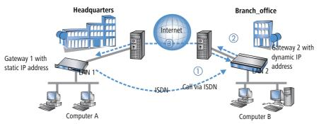
Gateway 1 calls Gateway 2 via ISDN. It takes advantage of the ISDN functionality of sending its own subscriber number via the D-channel free of charge. Gateway 2 determines the IP address of Gateway 1 from the preconfigured VPN remote stations using the received subscriber number.
