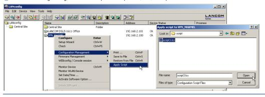
The upload of the script starts automatically. Status and error messages are either displayed directly by LANconfig or the can be viewed in a console session with the command show script.
