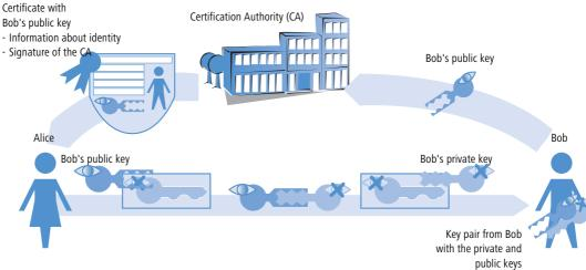
The certificate carries the signature of the CA to show that the confirmation itself is genuine. The certificate takes up just a small amount of data and is suitable for exchange with an asymmetric method. With a signature, however, the asymmetric method is used in the opposite direction:
