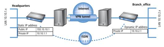
The VPN gateway **Branch office** initiates a VPN connection to the gateway **Headquarters**. **Branch office** has a dynamic IP address that was chosen and assigned by the Internet service provider upon dialling in, whereas **Head-quarters** has a fixed, static address. When the connection is set up, **Branch office** transmits its actual IP address to **Headquarters**. This is accomplished by a special ICMP packet (alternatively UDP, port 87).
