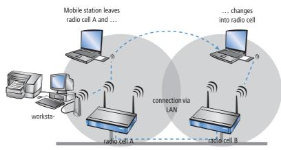
In the example above, the roaming function of the mobile station enables the access to the workstation in radio cell A also after changing into radio cell B. After the radio cell change, the base station in radio cell B passes on the data of the mobile station via LAN to the base station in radio cell A. From there, they arrive via radio at the workstation in radio cell A. In this way, the connection between both devices remains existing at any time.
