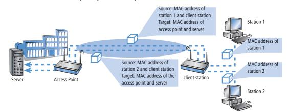
In this operating mode not the usual MAC addresses for instance in client mode are used (in this example for server, access points and client stations), but in conformity to point-to-point connections four addresses (the MAC address of the station in LAN of the client station is additional). The fully transparent connection of a LAN to the client station
