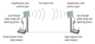
The calculation of the power over the path begins at the transmitters's radio module. The radio module in the LANCOM access points in 802.11a mode emits the following power levels depending on the channel used and the data transmission rate:
