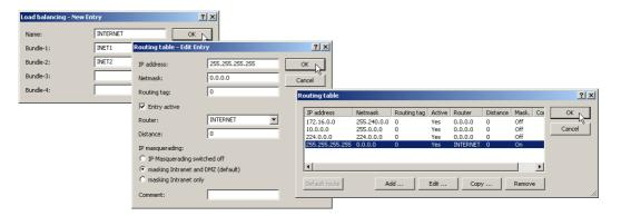
③ The virtual remote site is entered into the routing table as the router for the default route in LANconfig via IP router ► Routing ► Routing table.
