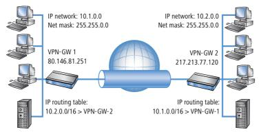
The description of the network relationships is more complicated if the source and target networks are not only represented by the intranet address ranges of the connected LANs:
