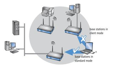
An Access Point in normal mode further clients can log on, but not in client mode.
