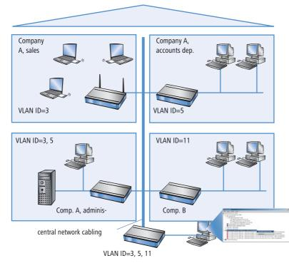
Virtual LANs enable to perform this task in a very smart way. Also when departments or companies change at a later time inside of the building, the network structure can be easily adjusted.
