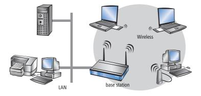
Larger exten- The area, in which mobile stations can get in touch with a base station, is called radio cell.
