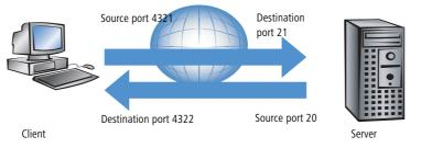
To enable this process, the administrator of the packet filter must open all ports for incoming connections, because he does not know in advance for which port the client will inquire the FTP connection. An alternative is to use passive FTP. Thereby, the client establishes the connection itself to the server over a particular port, which was told to the server before. This process is, however, not supported by all clients/servers.
