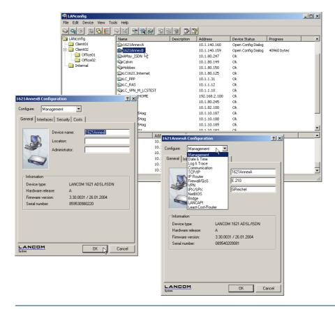
Cut and paste" can be used to transfer content between the configuration windows via the Windows clipboard.
