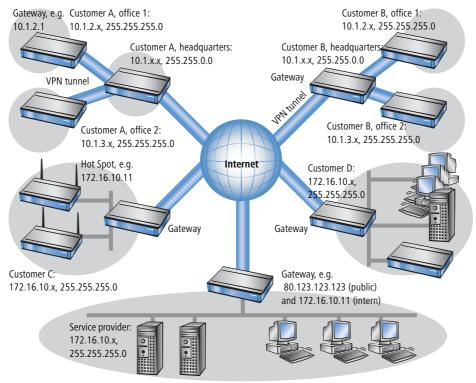
In this example, a service provider monitors the networks of different clients out of a central control. For this purpose, the SNMP-capable devices should send the respective traps of important events automatically to the SNMP trap addressee (e. g. LANmonitor) of the network of the service provider. So the LAN administrator of the service provider has an up-to-date view of the state of the devices at any time.
