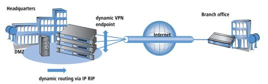
In decentralized company structures that rely on VPN for networking the various locations, the availability of the central VPN gateway is of particular significance. The company-wide communications only remain reliable as long as these central dial-in nodes are working properly.
