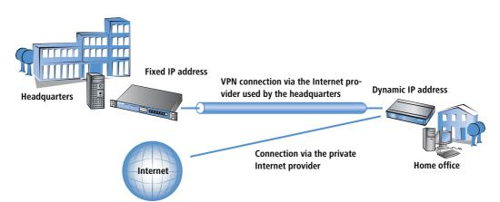
To ensure a clean separation of the data links, two Internet connections are established, one to each provider. In the IP routing table, the default route is assigned to the private provider; the network with the headquarters via the VPN connection is routed over the headquarters' provider.
