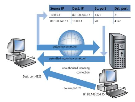
But if another workstation from the Internet tries to use the just opened port 4322 of the LAN to file itself data from its port 20 on the protected client, the Firewall will stop this try, because the IP address of the attacker does not fit to the permitted connection!
