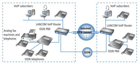
Along with data transfer via VPN, it is also possible to use VoIP functions between the two locations.
