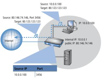
The response to this new packet is now sent to the IP address of the router with the new sender port number. The entry in the internal table allows the router to assign this response to the original sender again.
