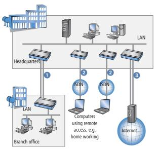
The corporate network is based on the internal network (LAN) in the headquarters. This LAN is connected to the outside world in three ways:
