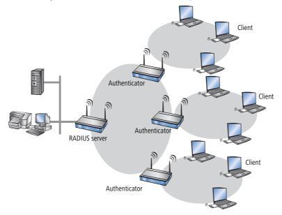
The authenticator has no initial information on the clients wanting to register. This is all stored in a database on the RADIUS server. The registration information the RADIUS server needs for the authentication process is stored in the database there and can vary from network to network. The authenticator has just the one task, that of transferring the information between the client and the RADIUS server.
