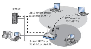
All requests with this protocol from this logical wireless network are automatically redirected to the target server in the LAN. The returning data packets are sent to the senders' addresses and ports according to the entries in the connection statistics, ensuring trouble-free operation in both directions.
