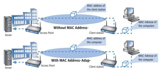
In some installations it is required, that the MAC address of the computer and not of the client station is transmitted. With the option Address-Adaption the replacement of the MAC address by the client stations is prevented and the data packets are transmitted with the original MAC address.
