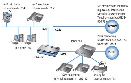
The LANCOM is operated on an ISDN PBX extension line.
