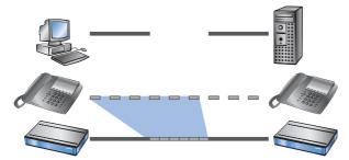
This annoying behavior can be compensated if all data packets, which are not belonging to the connection preferred by QoS, do not exceed a certain packet length. While doing so, the data packets of the FTP connection will be divided into such small sections that the time-critical VoIP connection is able to deliver the packets without noticeable delay within the required time slots. A resulting delay has no disadvantageous effect to the TCP-secured FTP transfer.
