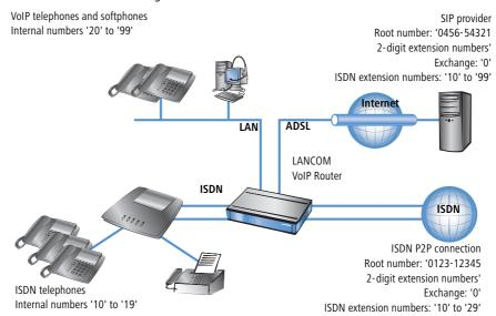
In this example we will take a look at a company planning to add a SIP trunking account, with up to 100 extension numbers, to its current ISDN point-to-point line having 20 extensions. The ISDN terminal devices with point-to-point line extensions used thus far can be retained. All new employees are to be issued with a SIP telephone with an extension via the SIP account.
