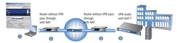
The two routers 2 and 3 have to permit the NAT-T connection between the two tunnel endpoints in that the firewall ports 500 and 4500 are activated, and port forwarding has to be activated in the terminating router at the headquarters, as well.
