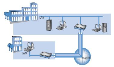
A VPN-enabled router (VPN gateway) is located at either end of the tunnel. The configuration of both VPN gateways must be matched to one another.
