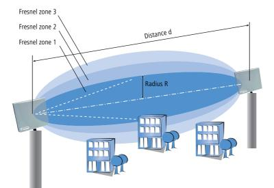
To ensure an optimal signal reception between transmitter and receiver, the Fresnel zone 1 should remain free from any obstruction. Any disturbances from elements protruding into this zone will significantly reduce the effective signal power. The object not only screens off a portion of the Fresnel zone, but the resulting reflections also lead to a significant reduction in the signal reception.
