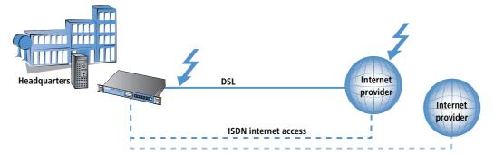
In this simple backup scenario, Internet access is realized via a DSL connection. An ISDN connection is defined as a backup in case of failure of the DSL Internet access.
