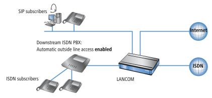
If the LANCOM VoIP Router in this constellation is not available, for example, due to a power outage, the ISDN connection for the downstream ISDN PBX is automatically "bridged" to the external ISDN connection (when life-line support is enabled). For a LANCOM VoIP Router **without** automatic outside line access, the ISDN subscribers should not dial a "0" before the number while the life-line support is active.
