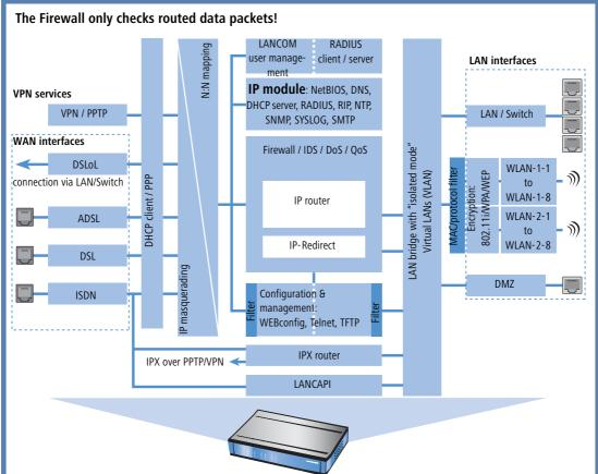
The Firewall only checks data packets routed by the IP router of the LANCOM. In general, these are the data packets, which are exchanged between one of the WAN interfaces and the internal networks (LAN, WLAN, DMZ).
