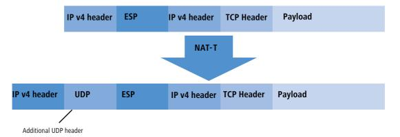
In order to use this process, both ends of the VPN connection (such as the WLANmonitor and a LANCOM router) have to use NAT-T.
