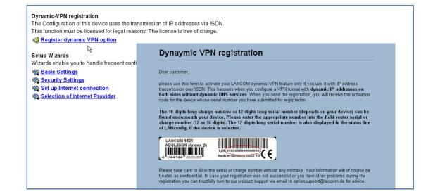
When using WEBconfig you can find a link on the first page which leads you to the registrating server of LANCOM Systems. There you must enter the serial number of your device and your e-mail address. After transmitting the data you receive a release code for the device.
