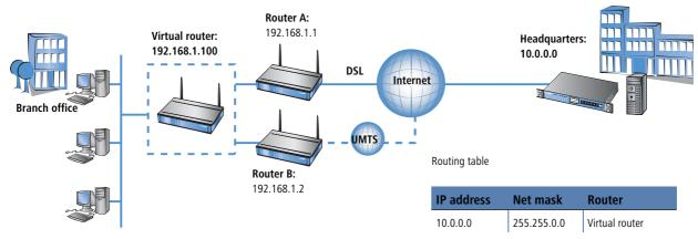
From a more technical standpoint, a router in a network requires a unique MAC address in addition to an IP address. Therefore, when defining a virtual router, a virtual MAC address is defined simultaneously which the virtual router reacts to. The virtual MAC address is formed as '00-00-54-00-01-xx', whereby 'xx' stands for the unique router ID.
