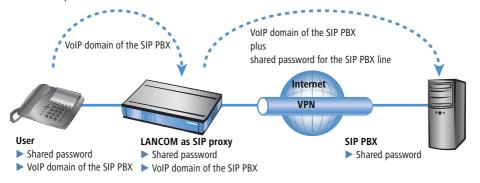
If SIP or ISDN users at the LANCOM VoIP Router are entered into the SIP PBX with different passwords, then the users have to enter their individual passwords upon registration. Consequently, each SIP or ISDN user has an entry into the LANCOM with the individual passwords, which are also entered into the SIP terminal devices. Users with shared and individual passwords can be managed in parallel.
