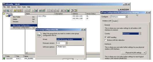
③ The parameters here should be set as required for the entire group. When the configuration dialogue is closed, LANconfig will request that you save the partial configuration file to a location of your choice.
