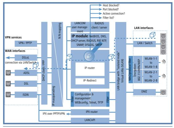
If no explicit Firewall rule exists for a data packet, the packet will be accepted ('Allow-All'). That grants a backward-compatibility for existing installations. For maximum protection by the Stateful Inspection, please note the section 'Set-up of an explicit "Deny All" strategy'  $\rightarrow$  page 199.
