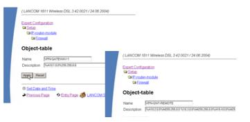
Under Configuration > Firewall/QoS > Rules table define a new firewall rule named "VPN-GW1-OUT". Set the objects to "CPN-GW1-LOCAL" and "VPN-GW1-REMOTE", the protocol to "ANY" and the action to "ACCEPT". Activate the option "VPN rule" so that the IP networks described in this rule will be used in establishing VPN network relationships.
