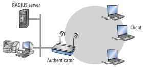
Authentication server: RADIUS server on which user data is configured. This is usually located within the same network for which it issues access authorizations. It is accessible to the client via the authenticator. Some scenarios may also allow the use of a LANCOM access point for this task.
