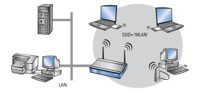
In some applications, however, it may be desirable to divide the clients the radio cell into different groups, each of which is treated in a certain way by the access point. It may be necessary, for example, to operate a public wireless network without any encryption simultaneous to a protected, 802.11i-, WPA- or WEP-encrypted wireless network that excludes unauthorized parties.
