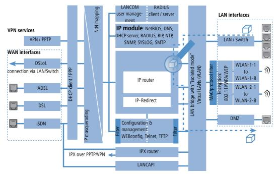
A direct data exchange between LAN and DMZ via LAN bridge is not possible if a dedicated DMZ port is used. The path from LAN to DMZ and vice versa is therefore only possible through the router, and thus also only through the Firewall! This shields the LAN against inquiries from the DMZ, similar to the LAN against inquiries from the Internet.
