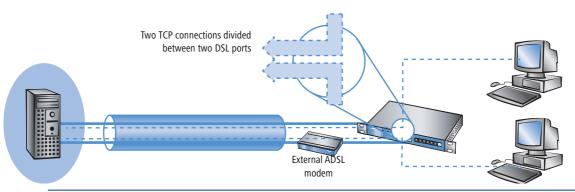
Unlike direct channel bundling, load balancing offers the true sum of all bundled bandwidths. This version is thus highly effective for combining different bandwidths.
