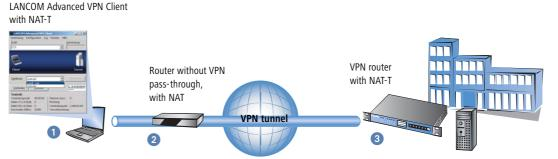
Both tunnel end points LANCOM Advanced VPN Client 1 and VPN router 3 support NAT-T and can therefore also establish a VPN connection through the intermediary router.
