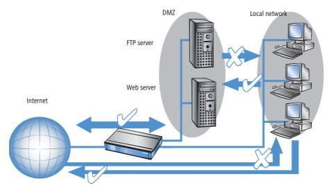
Some LANCOM models support this structure by a separate LAN interface only used for the DMZ. Looking at the path of data through the LANCOM, then the function of the Firewall for shielding the LAN against the DMZ becomes visible.
