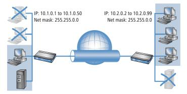
In many network structures, the local network is connected by further routers to sections of other networks with their own IP address ranges. Additional settings are required to include these address ranges in the network relationship.
