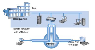
The VPN gateway of the LAN must support the establishment of VPN tunnels with the VPN client software of the remote PC.
