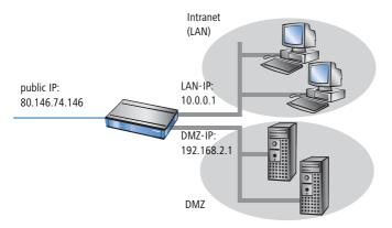
The option **Masq.** in the Service list informs the router, if the local intranet or DMZ addresses should be hidden behind the IP address of the router:
