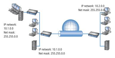
In these cases, the network relationships that describe the source and target networks must be entered manually. Depending on the situation, the scope of the automatically generated VPN rules may be extended, although sometimes it is better to deactivate the automatic VPN system to prevent unwanted network relationships.
