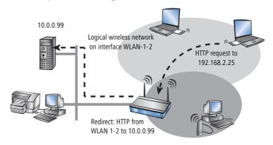
All requests with this protocol from this logical wireless network will automatically be redirected to the target server in the LAN. The returning data packets are sent to the senders' addresses and ports according to the entries in the connection statistics, which ensures the trouble-free operation in both directions. Further information to the configuration of the protocol filter can be found 'Protocol filter'  $\rightarrow$  page 359
