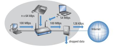
To solve this problem, the transfer rate of the LANCOM's WAN interface will be reduced artificially. This interface will thereby be adjusted to the transfer rate that is available for the actual data transport towards the WAN. For a standard DSL connection, the DSL interface is thus adjusted in the LANCOM to the appropriate upstream rate (e.g. 128 kbps).
