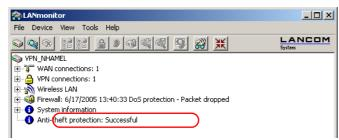
With WEBconfig (Expert Configuration > Status > Config > Anti-Theft-Protection) or Telnet (Status/Config/Anti-Theft-Protection) you can also look up the ISDN Location Check.
