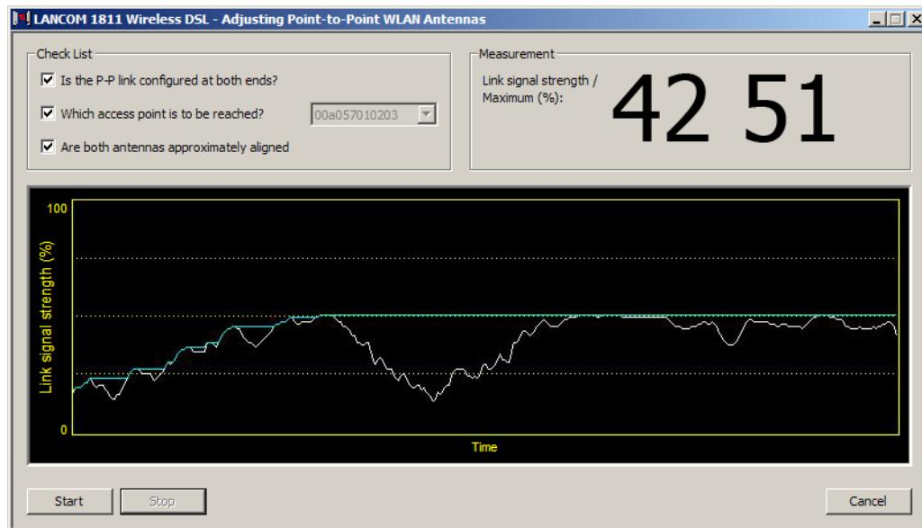
Initially you should only adjust one of the two antennas until a maximum value is achieved. This first antenna is then fixed and the second antenna is then adjusted to attain the best signal quality.
