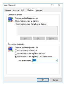
In Firewall / Qos > IPv6 Rules > IPv6 forwarding rulesyou can create a new rule. Entries from the DNS destinations or DNS destination list tables can be used as Target stations.
