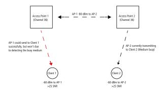
An access point can be set artificially "deaf" by reducing the reception sensitivity from LCOS 10.30 RU1 onwards. This means that transmissions further away from the access point are "overheard" and the channel is detected more often as "free". In simplified terms, more simultaneous transmissions on the same channel are possible. On the one hand, this increases the overall throughput of a system, but on the other hand, the interference on the client side also increases.
