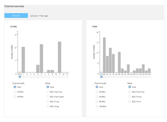
The two bar charts visualize how many SSIDs the device detected on the various 2.4- and 5 GHz channels, which can represent the potential load on the channels.
