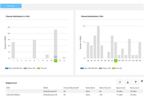
Click the button **Start scan** to discover the WLAN environment. After the scan is completed (duration: approx. 10 seconds), the results are shown in various diagrams and tables:
