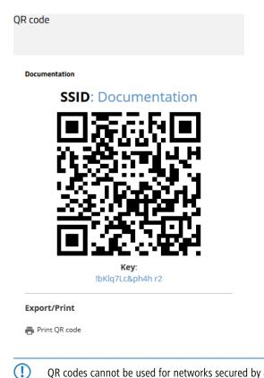
QR codes cannot be used for networks secured by 802.1X as they do not use a static WLAN key (PSK).
