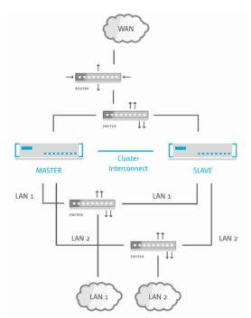
The following figure illustrates a typical network environment with a redundant master/slave configuration for High Availability.
