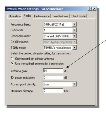
By setting the antenna gain, the output power is automatically adopted to the maximum power (referring to country, data rate and frequency band).
