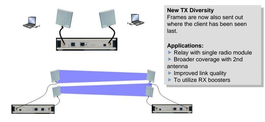
Standard Antenna Diversity: Frames are received always by the antenna that is nearest to the client, while being sent out always on the main antenna.
